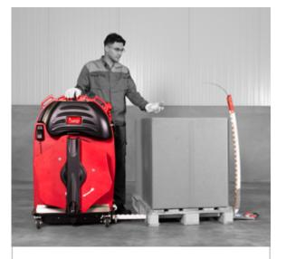
Roll the **ErgoStrap** in front of the pallet. The ChainLance pulls the **strap** through under the pallet.
